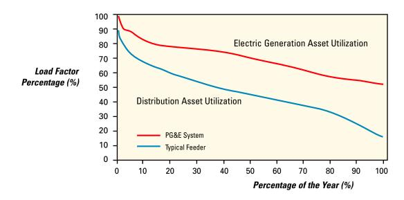
**Figure 2.** *Comparison of load duration curves for a distribution feeder vs. generation*<sup>26</sup>
