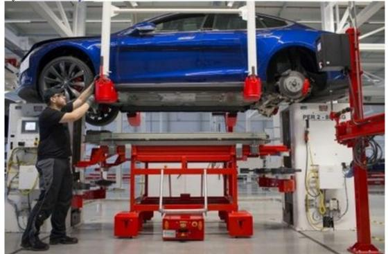
An employee positions a Tesla Model S automobile during the battery-pack fitting on the final assembly at a Tesla factory in Tilburg, Netherlands, in 2015. (Jasper Juinen/Bloomberg)
