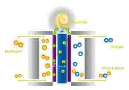
Fuel cells don't burn hydrogen - they use an electrochemical process to convert hydrogen and atmospheric oxygen into electricity and water. They have no moving parts and no open flames.
