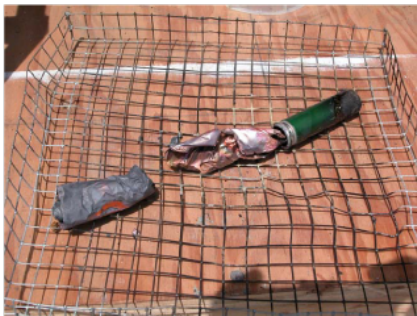
FIGURE 5. EXPLODED CELL AND ITS CONTENTS
