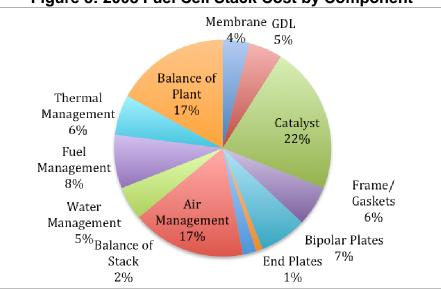
Figure 3: 2008 Fuel Cell Stack Cost by Component
