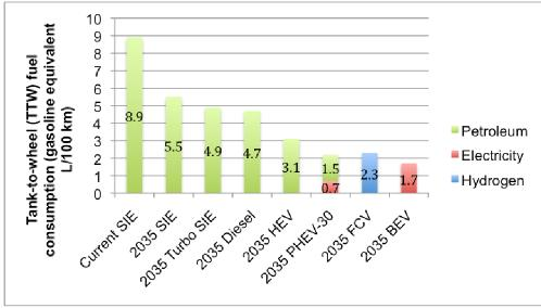
Figure 1: Tank-To-Wheel Gasoline Equivalent Fuel Consumption
