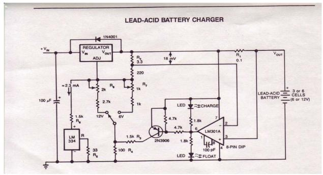
Figure 8: Lead-Acid Battery Charger Circuit Diagram
