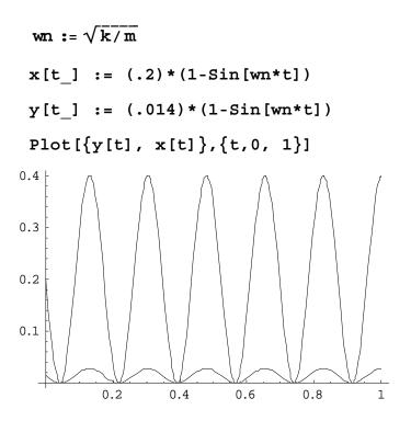
The above graph shows that the ASTM standards require a much higher displacement of the stack than the standards of the stack specify. However, this is a very preliminary vibration analysis. It does not account for the fact that the stack can withstand a constant acceleration of 5g from 60Hz to 150Hz, which is much higher than the 7 Hz vibrations that the ASTM standards specify.
