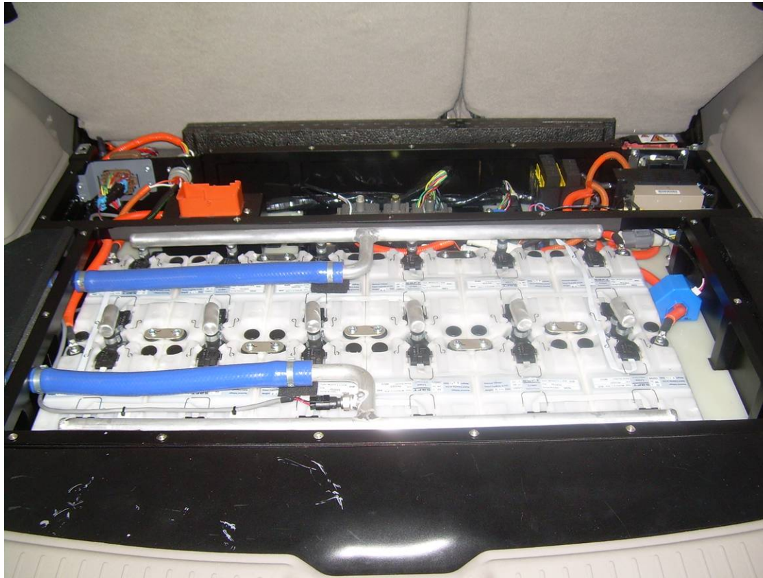
Final PHEV HV Battery Integrated Into vehicles
