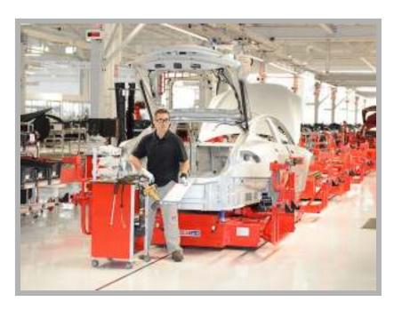
Magnetic strips laid onto the floor guide the Smart Carts. This gives Tesla great flexibility to reconfigure the layout for other models in the future.
