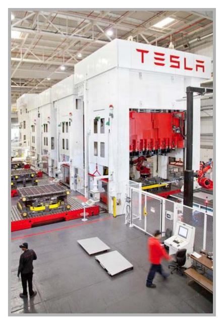
Tesla produces 95 percent of the parts in-house. Huge stamping presses produce aluminum body panels. Resin injection molding machines and die casting create aluminum components. The imported AA-size battery cells—more than 7000 are used in each battery pack—are assembled into the battery packs on the second floor.
