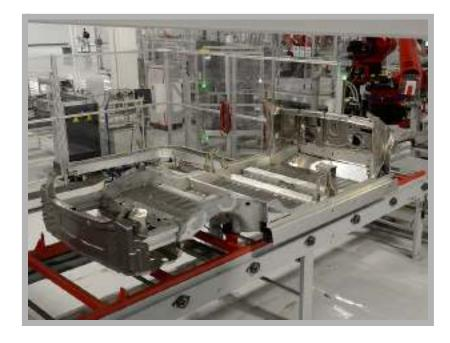
A completed floor pan shows how aluminum castings, aluminum stampings, and high-strength steel are bonded, welded, and riveted together to make a strong but lightweight structure.
