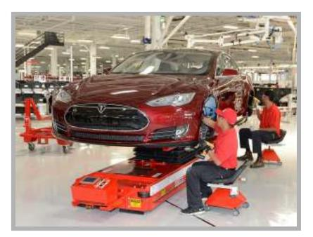
Smart Carts, rather than a fixed assembly line, carry the Model S bodies around the factory during final assembly. The body can be raised or lowered to make it easier for Tesla workers.
