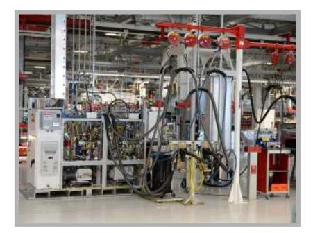
This array of hoses and tubes puts the fluids into the cars near the end of the production line, just before they go through a final quality-control check on an indoor test track.
