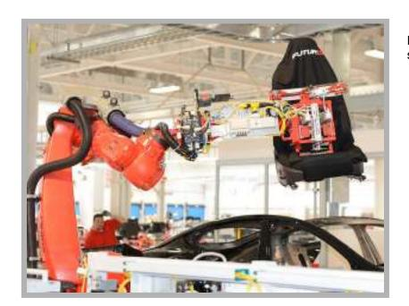
Robots install the Model S seats.
