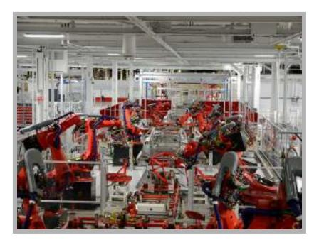
Tesla removed all the old assembly equipment and installed new robots that can perform several different functions, such as assembling the chassis. Some robots are true multitaskers that can weld, rivet, glue, and lasercut.
